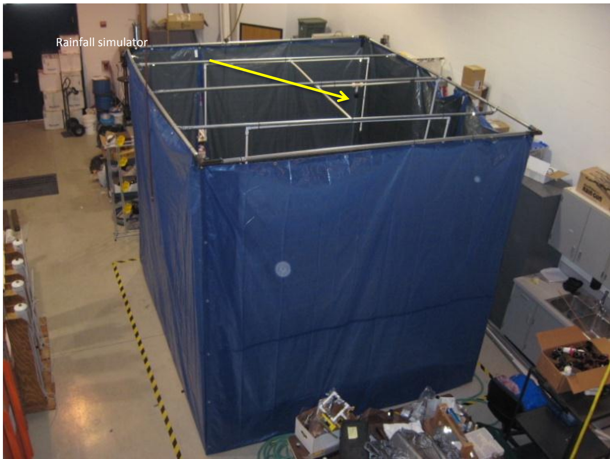
Figure 2-3. Rainfall simulation system for the laboratory runoff experiment
