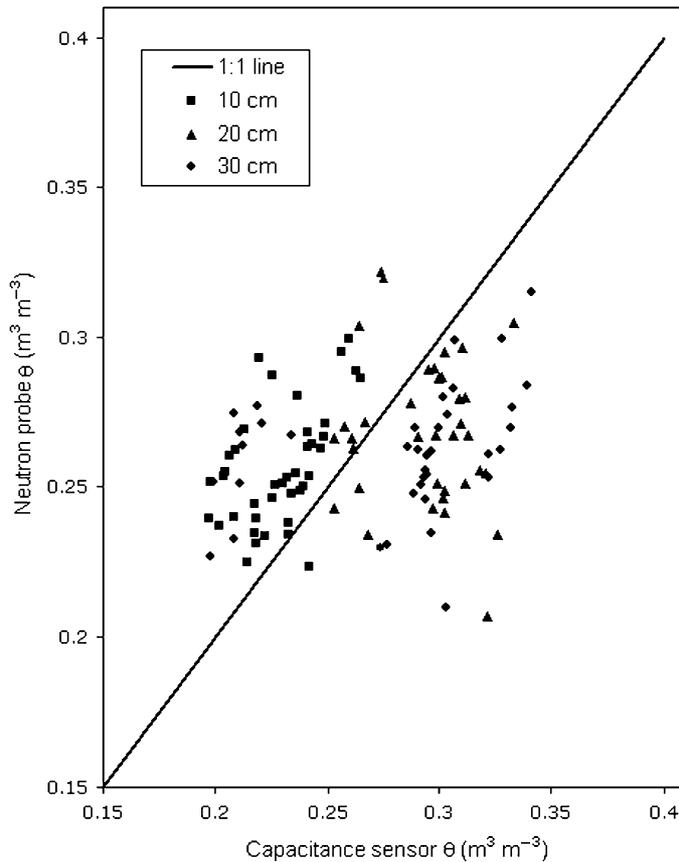
Fig. 5. Comparison of volumetric soil-water content ( $\theta$ ) of Krome calcareous very gravelly loam soil in an orchard determined with a neutron probe and capacitance sensors showing the deviation for a 1:1 correlation line for data collected at 10, 20, and 30 cm below the soil surface.
