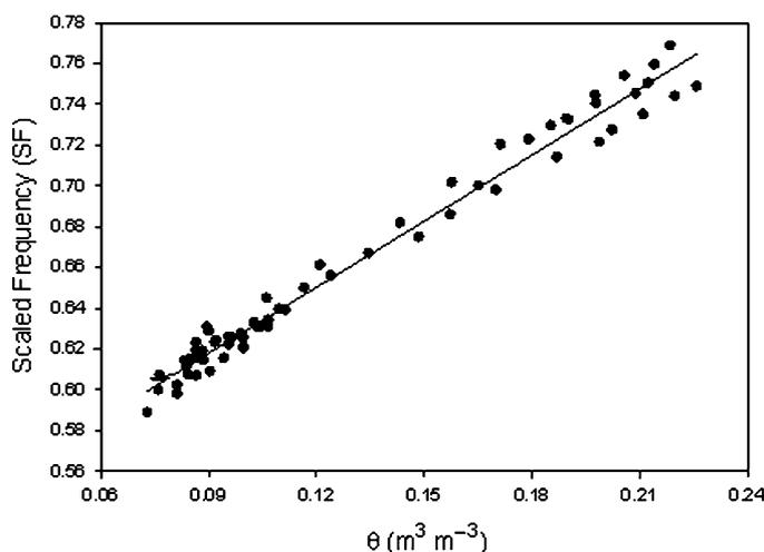
Fig. 1. Relationship between scaled frequency (SF) from a multi-sensor capacitance probe (EnviroSCAN) and volumetric water content ( $\theta$ ) fitted to obtain calibration coefficients for Krome calcareous very gravely loam soil in containers,  $y = 0.011x + 0.5206$ ;  $r^2 = 0.98$ .
