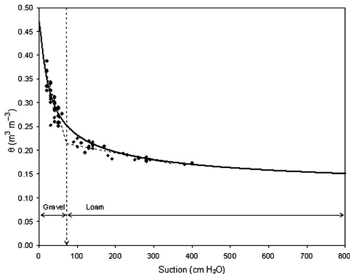
Fig. 3. Soil-water characteristic curve for Krome calcareous very gravelly loam soil collected from fallow vegetable fields. Suction and volumetric soil-water content ( $\theta$ ) were determined with pressure cells and a pressure plate in the laboratory and the curve was fit with van Genuchten's (1980) model.
