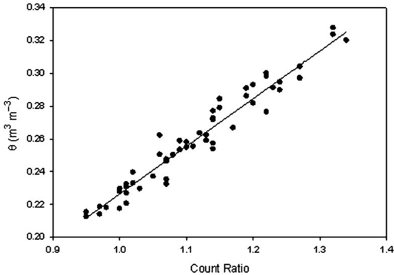
Fig. 2. Relationship between count ratio from the neutron probe and volumetric water content ( $\theta$ ) fitted to obtain a calibration equation for Krome calcareous very gravelly loam soil in containers,  $y = 29.05x - 6.4$ ;  $r^2 = 0.95$ .
