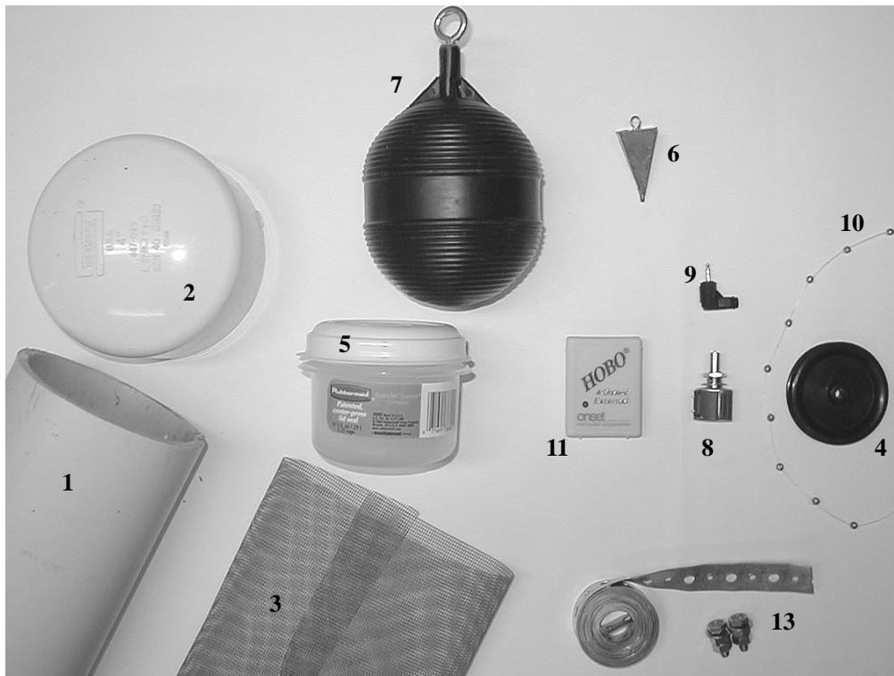
Figure 1. Materials used in the construction of the stage recorder. Numbers correspond to those given in table 1 (item 12 not pictured).
