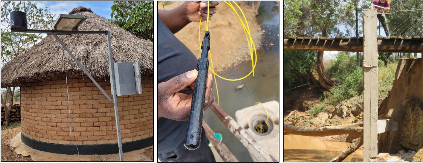
Figure 3-5. Monitoring equipment in Laikipia, Kenya. Left: Rainwise tipping bucket rain gauge with solar panel and battery box. Center: Solinst Levelogger 5 with direct read cable removed from streamgage housing below. Right: Streamgage housing visible from dry river conditions. Concrete box contains metal pipe interior and was constructed on site, with locks at top crafted by local metalworker to reduce possibility of theft. Photos courtesy of author.
