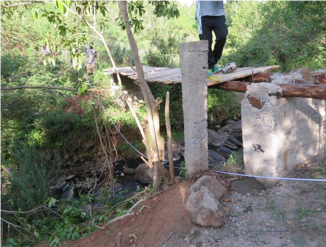
Figure B-2. Timau – CA02 streamgauge from downstream right bank looking upstream. Similar to CA01, this gauge location is only responsive to high rainfall and installation was limited by bedrock. Photo courtesy of author.
