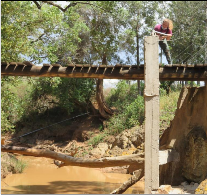
Figure B-3. Storms Bridge – CA03 streamgage from downstream looking upstream. This gauge is subject to very ‘flashy’ streamflows and is shown here during low-flow conditions. Photo courtesy of author.
