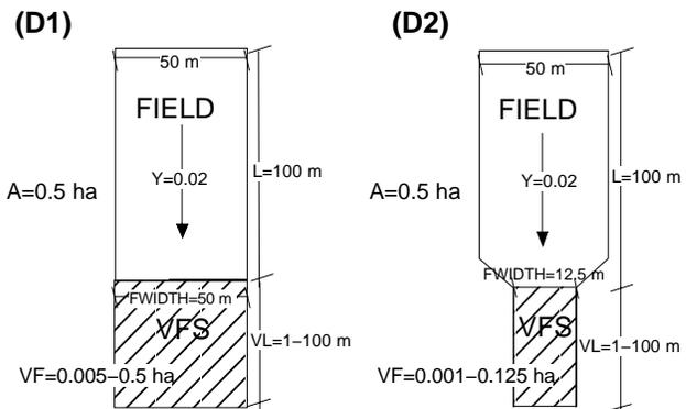
Figure 2. Design alternatives for different filter to buffer area ratios (not to scale, labels described in table 3).
