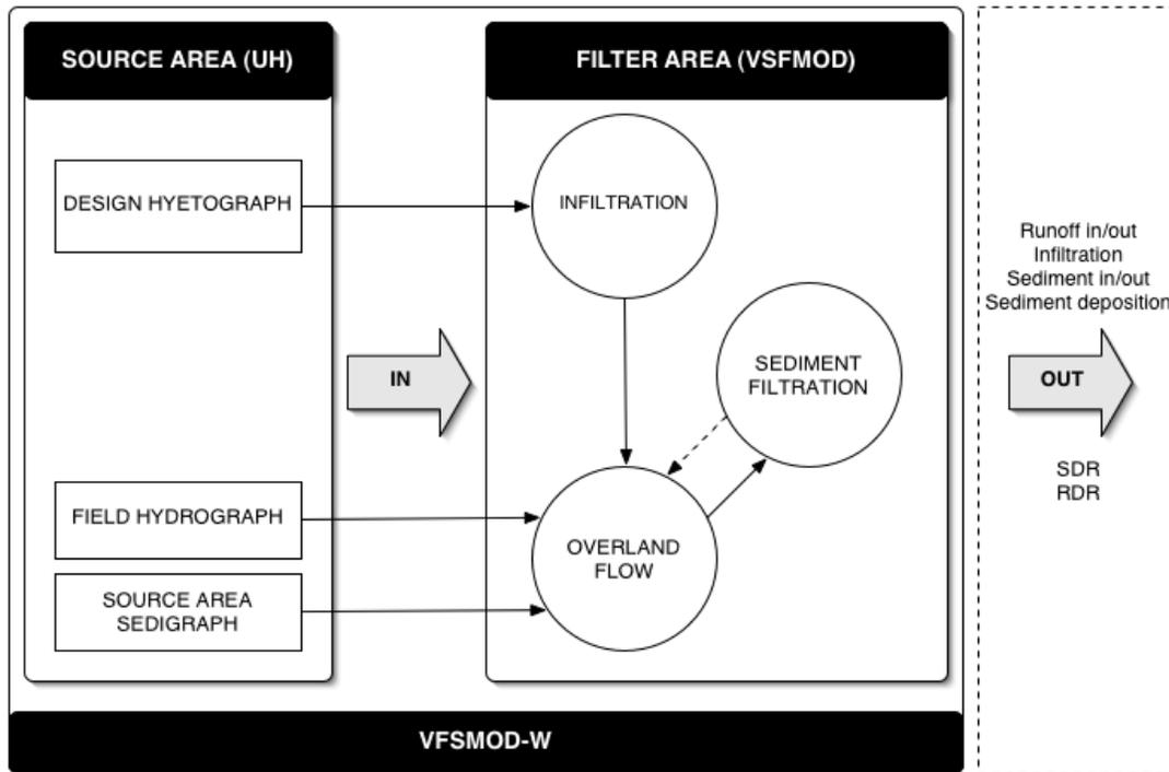
Figure 1. Schematics of the combined model (VFSMOD-W) for vegetative filter strip design.
