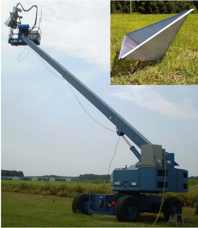
Fig. 1. UF-LARS mounted on the 25 m Genie platform. (Inset) Trihedral calibration target made of aluminum.
