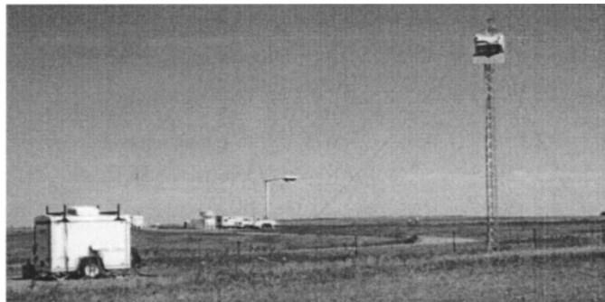
Fig. 2. Picture showing TMRS setup at the ARM-CART Central Facility near Lamont, OK. A truck-based microwave system with L-, S- and C-band radiometers from NASA Goddard Space Flight Center can be seen in the background.
