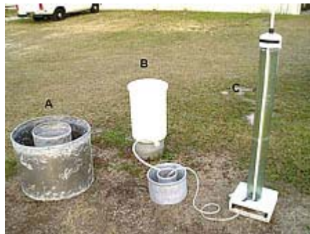
Fig. 1. Photograph of (A) 30-cm diameter (inner) and 60-cm diameter (outer) double-ring infiltrometer (B) 15-cm diameter (inner) and 30-cm diameter (outer) double-ring infiltrometer, and (C) Mariotte siphon developed to maintain a constant inner head in the infiltration rings.
