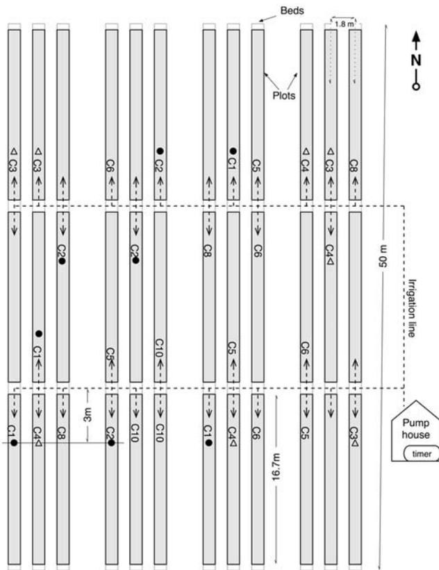
**Figure 5.** Tomato field layout used to test the QIC controller (not drawn to scale). Beds are divided into three irrigation plots, each controlled by independent solenoid valves (arrows). Each unit is a replication for the corresponding irrigation treatment (C1-C10). Replications for treatments C1-C4 have soil water sensors buried 3 m from the solenoid valve with controllers wired in closed-loop with the timer at the pump house (● switching tensiometers; ▽ QIC/capacitance probes).
