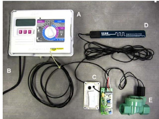
Figure 3. Details of a time clock irrigation control system retrofitted with the soil water sensor and showing: (A) time-based controller, (B) external power supply, (C) Quantified Irrigation Controller circuitry, (D) capacitance soil water probe (ECH<sub>2</sub>O, Decagon Devices, Inc., Pullman, Wash.), and (E) solenoid valve.
