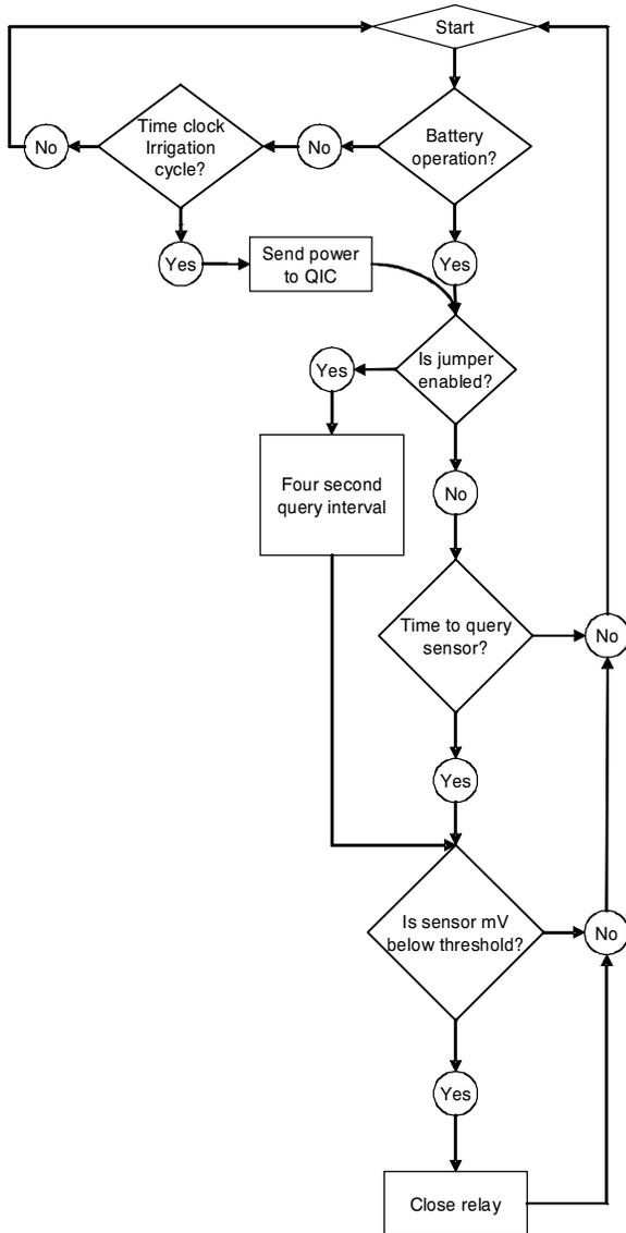
Figure 2. Quantified Irrigation Controller decision logic flowchart. The relay is normally open (closed valve position).
