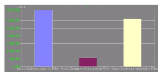
(b) Mass Sediment Input to Filter, Mass Sediment Output from Filter, Mass Sediment retained in Filter Under the Given Rainfall and VFS Width Condition
