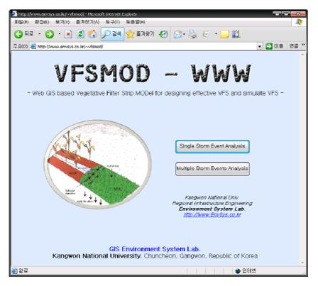
Fig. 4. Single Storm Event and Multiple Storm Events Analysis Options in the Web GIS based VFSMOD System (http://www.EnvSys.co.kr/~vfsmod)
