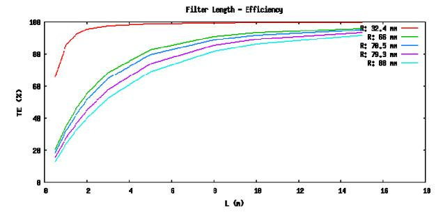
Fig. 14. Trapping Efficiency under Various Design Storm Event and Filter Strip Width Conditions - Multiple Storm Events Analysis Output Interface of the Web GIS based VFSMOD System
