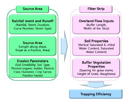
Fig. 2. Input data of Source Area and Filter Strip Component of the VFSMOD
