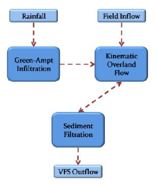
Fig. 3. Overview of sub-modules in VFSMOD-w
