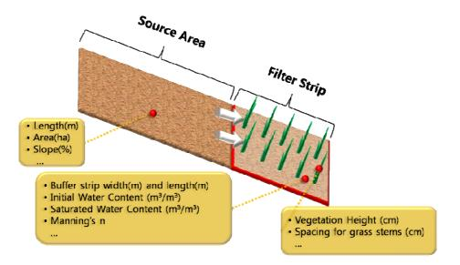
Fig. 1. Source area and Filter strip in VFSMOD-w
