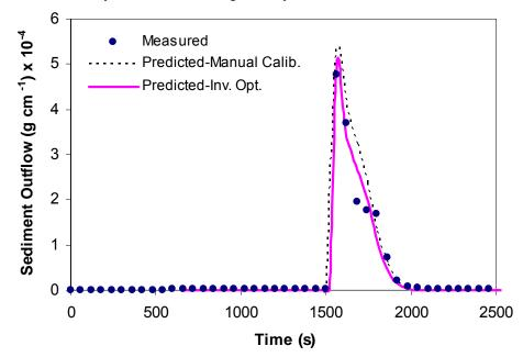
Figure 6. Example of VFSMOD-W performance using the sediment component parameters obtained by inverse modeling and by manual calibration.
