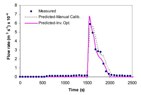
Figure 5. Example of VFSMOD-W performance using the flow component parameters obtained by inverse modeling and by manual calibration.
