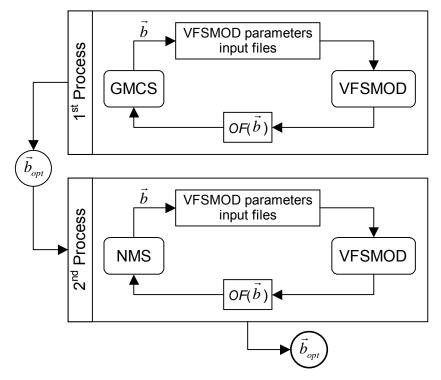
Figure 1. Scheme for the inverse modeling procedure to calibrate the VFSMOD parameters
