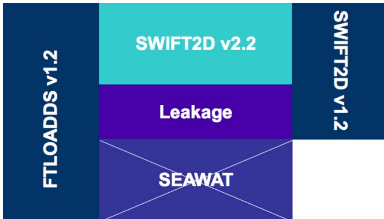
Figure A-5. FTLOADDS v1.2 comprises SWIFT2D v2.2 with updates for TIME but with the ground-water simulation turned off (thus SWIFT2D v1.2).
