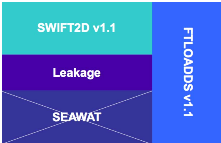
Figure A-2. FTLOADDS v1.1 comprises the SWIFT2D v1.1. code, leakage code linking SWIFT2D to SEAWAT, and SEAWAT, but represents applications in which SEAWAT is not implemented.
