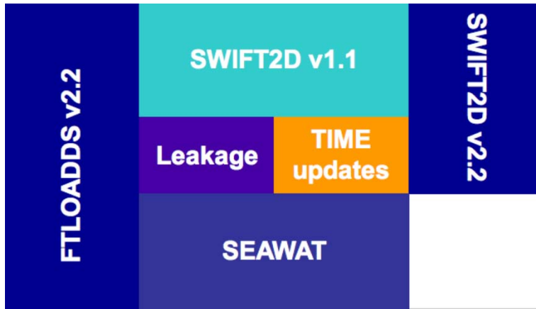
Figure A-6. FTLOADDS v2.2 contains SWIFT2D v2.1 linked with SEAWAT and containing TIME updates (thus SWIFT2D v2.2).
