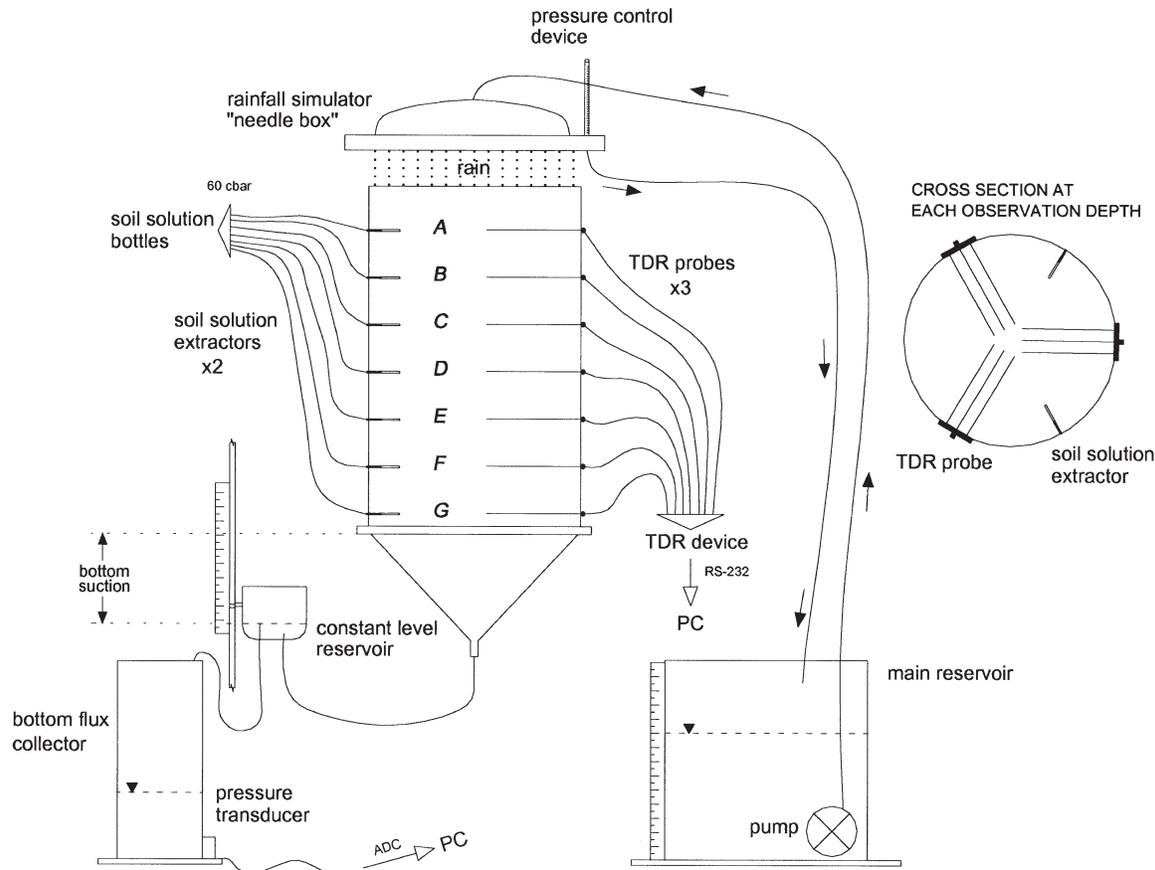
Fig. 1. Experimental set-up for transport experiments in the volcanic soil monolith.
