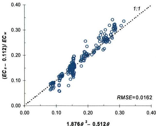
Fig. 3. Correlation between values measured in the suction extractor samples and estimations obtained with the TDR.
