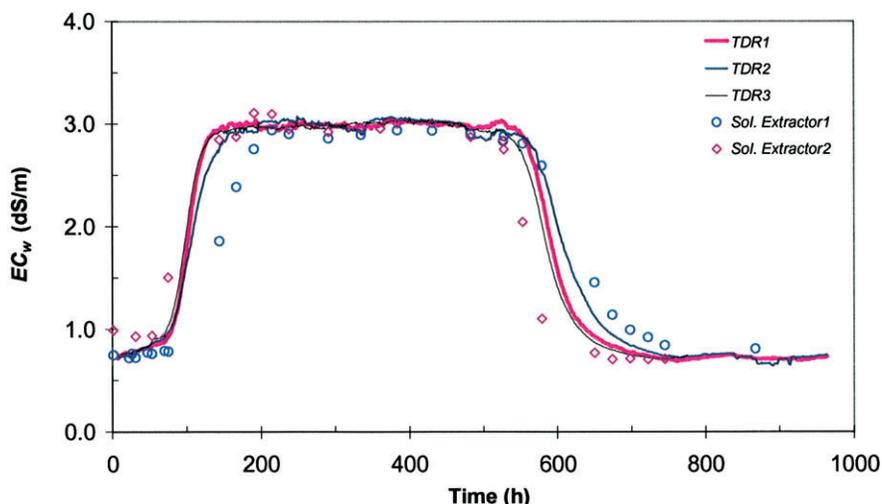
Fig. 2. Breakthrough curves observed at the middle of the monolith (Depth D) by TDR (lines) and solution extractors (each with a different symbol).
