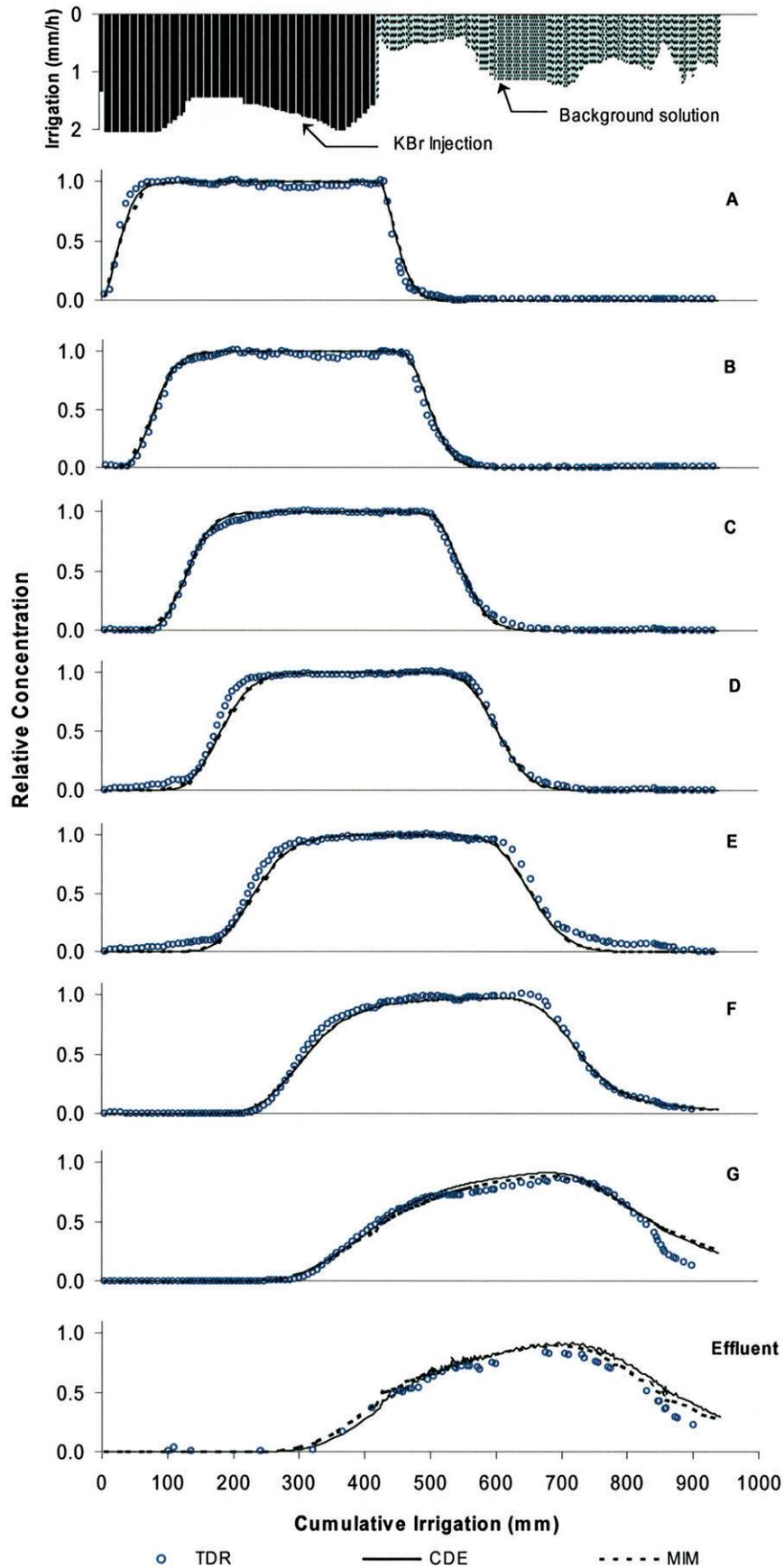
Fig. 4. Average breakthrough curves at the seven observation depths and on effluent. Breakthrough curves were obtained from TDR (symbols) and simulated by the WAVE model with CDE (solid lines), and with MIM (dashed lines).
