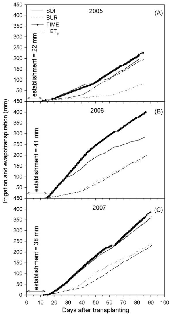
**Fig. 2 – Cumulative irrigation and estimated evapotranspiration (ET<sub>c</sub>) after initial plant establishment as affected by different irrigation scheduling methods during the 2005, 2006, 2007 tomato growth season.**
