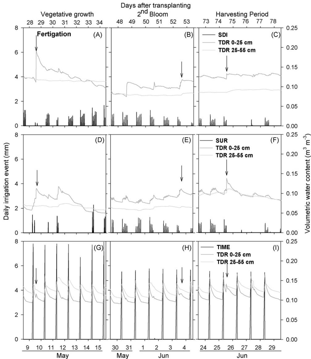
**Fig. 4 – Daily irrigation events and volumetric soil water content (0–25 and 25–55 cm depth) for tomato during three crop development stages (vegetative growth, 2nd bloom and harvesting period) during the spring of 2006 for SDI (A–C), SUR (D–F), and TIME (G–I) treatment. The arrows indicate fertigation events.**
