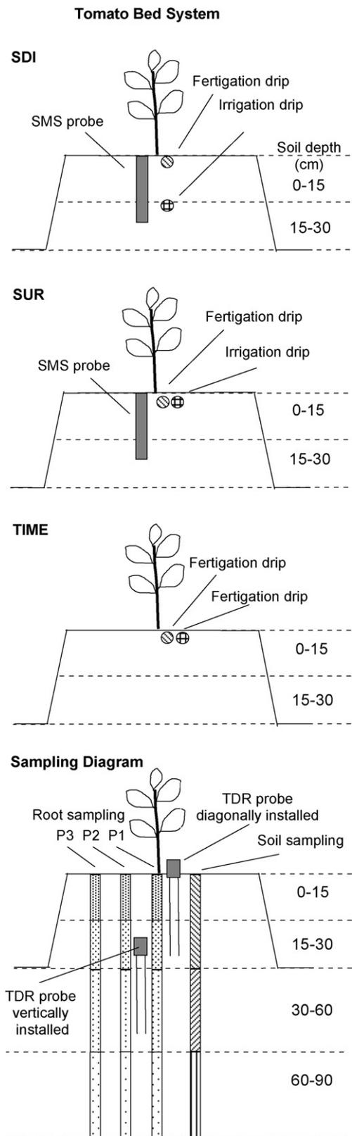
Fig. 1 – Overview of irrigation drip system, soil moisture sensor (SMS) placement and sampling scheme.
