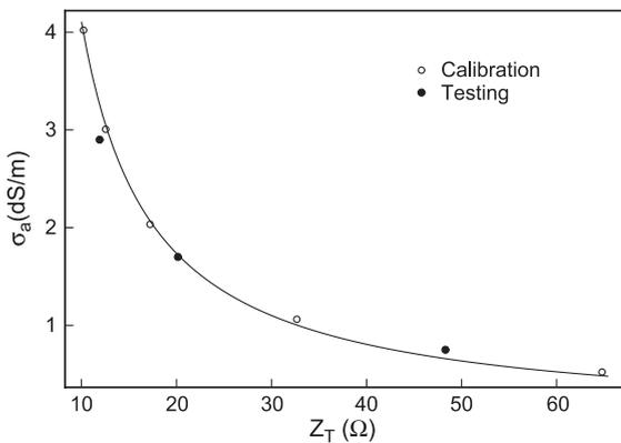
Fig. 5. Experimental fitting of Nadler’s model (Eq. (6)) ( $K_c=30.06$ ,  $Z_{\text{cable}}=2.68 \text{ } \Omega$ ) to estimate the electrical conductivity of five KCl reference solutions.
