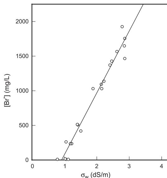
Fig. 9. Relationship between  $[\text{Br}^-]$  tracer concentration and soil solution electrical conductivity.
