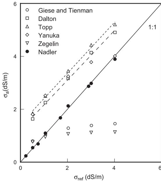
Fig. 4. Experimental comparison of TDR equations to estimate the electrical conductivity of five KCl reference solutions.
