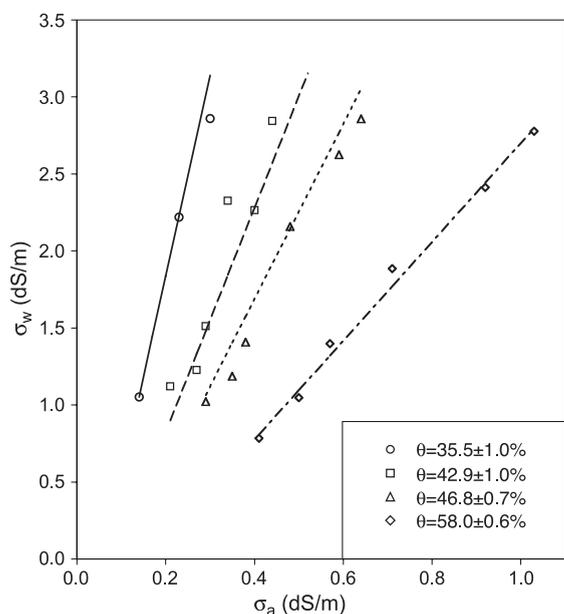
Fig. 8. Performance of proposed alternative empirical model with experimental TDR data from this study and New Zealand soils.
