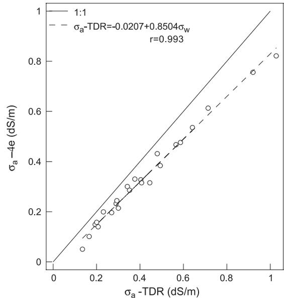
Fig. 6. Comparison of instruments to estimate soil  $\sigma_a$ .
