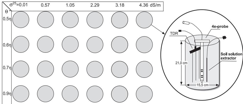
Fig. 2. Experimental set-up for calibrating soil electrical conductivity models.
