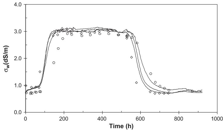
Fig. 10. Comparison of breakthrough curves obtained at the center of the soil column using TDR (lines) and solution extractors (symbols).
