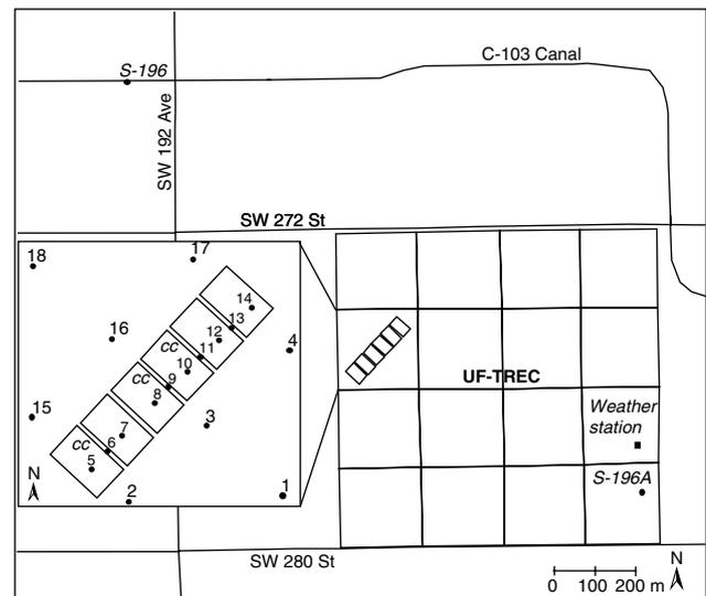
Figure 1. Location of experimental site at UF-TREC showing canal C-103 with the SFWMD's S-196 canal recording gated culvert (upper left corner), and the USGS' S-196A recording well next to the automatic weather station (lower right corner). Each square of the grid represents a 4-ha research field (200 by 200 m). The inset depicts the location of the 18 sampling wells and the corn crop strip along the diagonal (six rectangles). Plots marked with 'CC' used Sunn Hemp as summer cover crop
