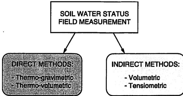
FIGURE 5.1 Methods for measuring soil moisture.
