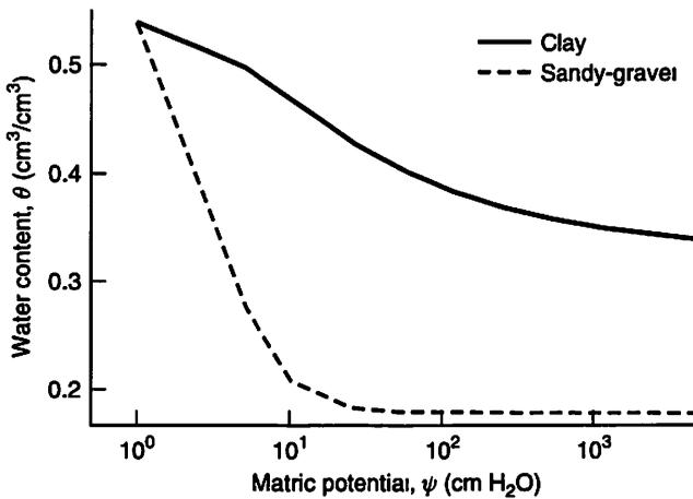
FIGURE 5.2 Measured soil water characteristic curves for two different soil types.
