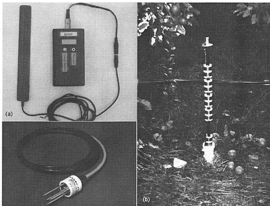
FIGURE 5.5 FD probes: (a) capacitance; (b) FDR.
