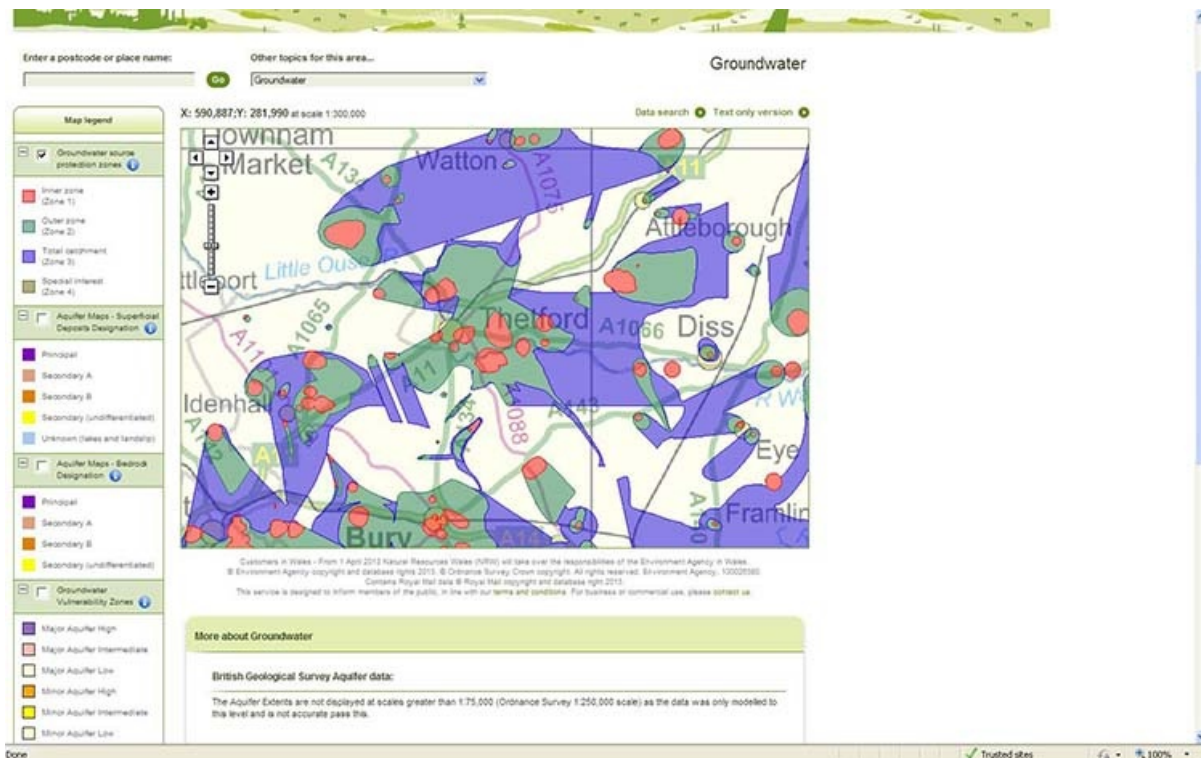
Figure 5.7: Illustration of the source protection zones defined by the Environment Agency to protect groundwater sources (EA 2013d).
