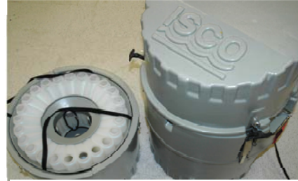
Water sampler with 24 bottles for sampling runoff water
