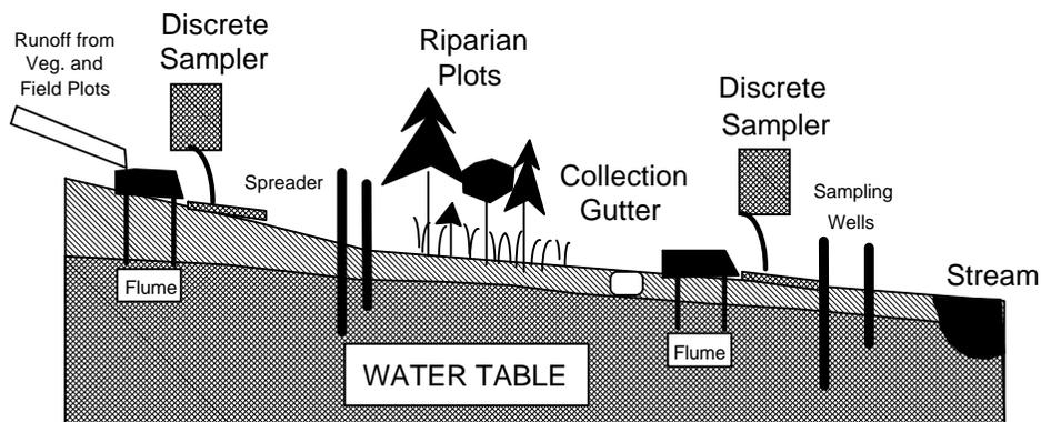
Figure 4. Details of surface water collection system in the riparian areas.
