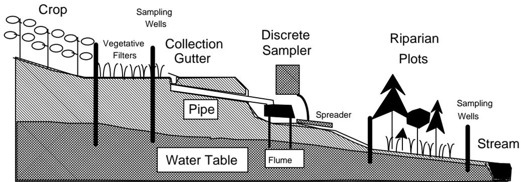
Figure 3. Schematic of surface water quality collection system from the grass filters and the field edge.
