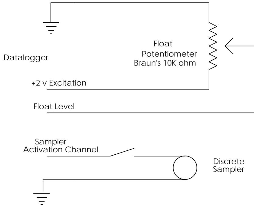
Figure 6. Details of Datalogger hookup for float measurements and sampler activation.
