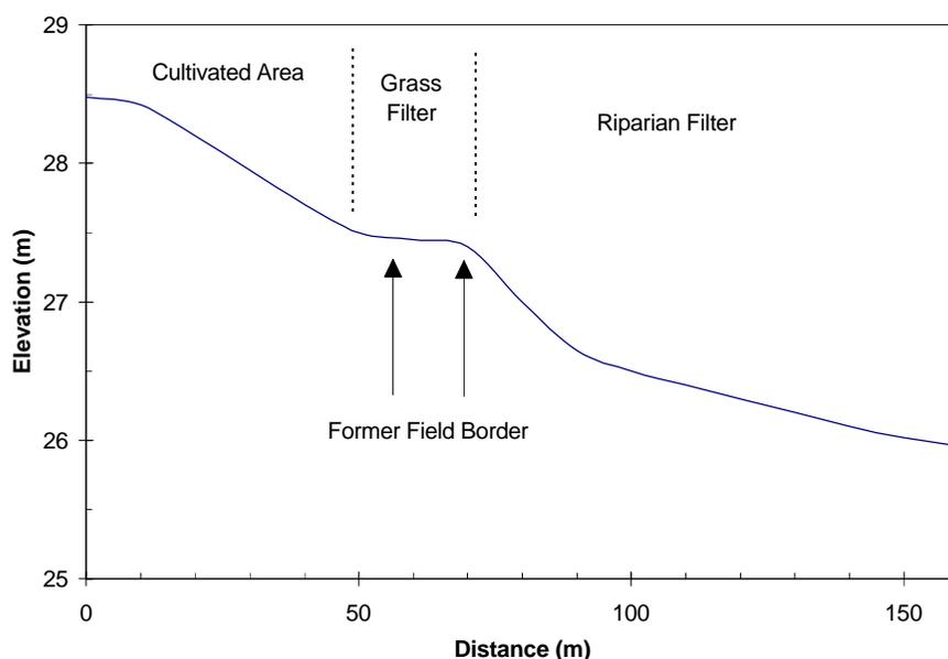
Figure 1. Cross-section of Coastal Plain site showing the relative slopes in the cultivated, grass filter and riparian filters. The Piedmont site is similar except slopes in the forested filter plots are about 12%.
