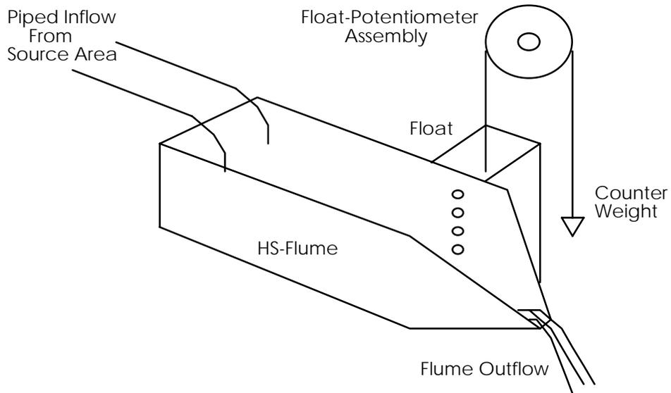
Figure 5. Flume showing the potentiometer-float measurement assembly.
