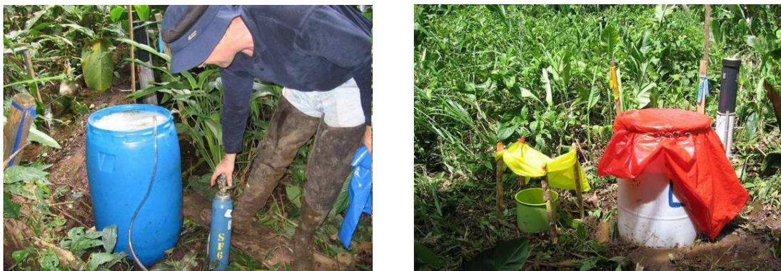
Figure 11: SF<sub>6</sub> sparging (left) and barrel with its reference bucket (right; under yellow plastic).
