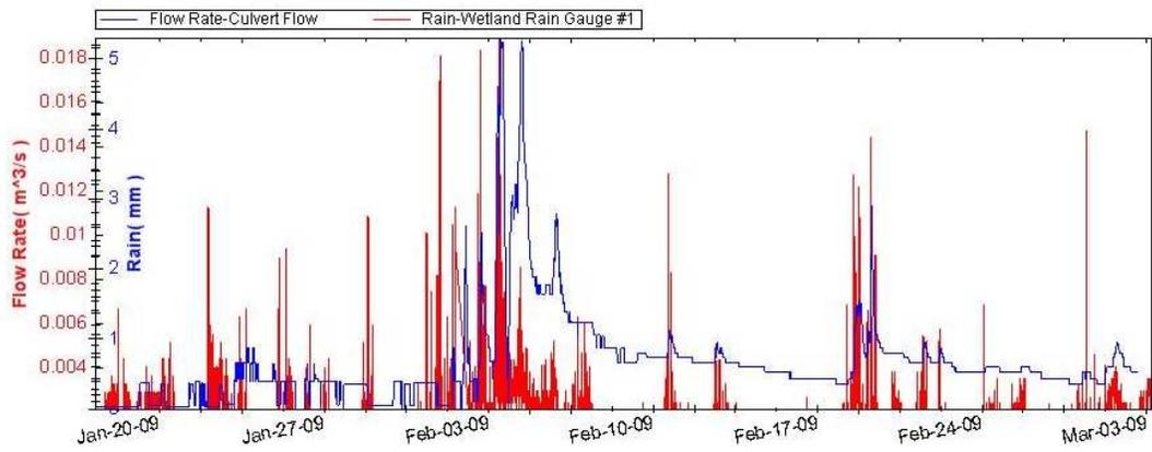
Figure33: 15-min flow data ( $m^3/s$ ) with 5-min rainfall data from January 19<sup>th</sup> to March 4<sup>th</sup>.
