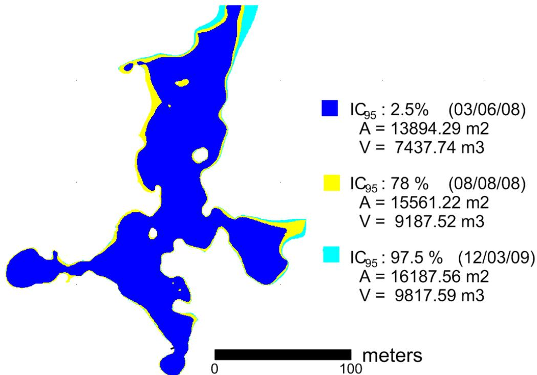
Figure 7: Overlay of three daily water surface representing the most frequent water area (yellow) with the lower (dark blue) and the upper (light blue) boundary of the 95% confidence interval of the frequency distribution.
