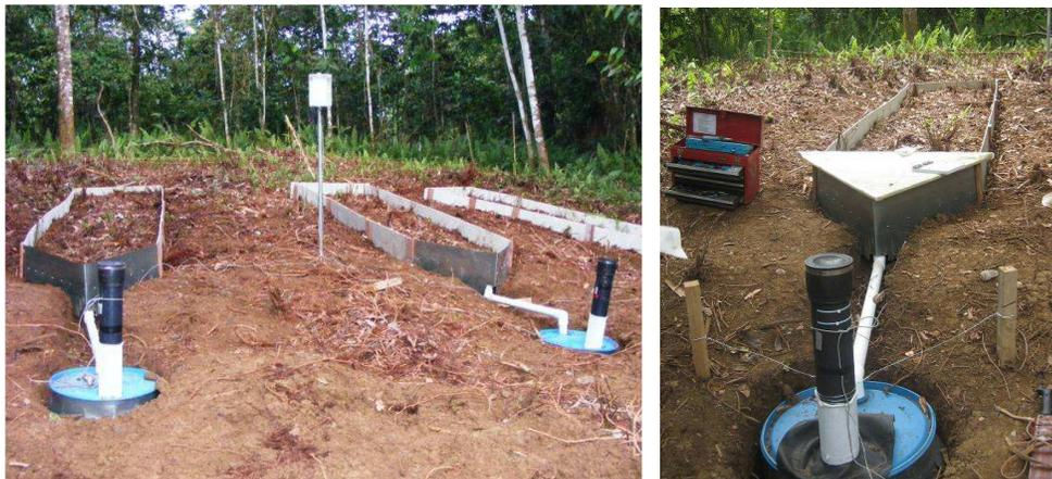
*Runoff plots with water stage recorders in blue barrels.*
