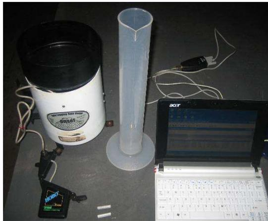
*Calibration kit with two types of nozzles.*
