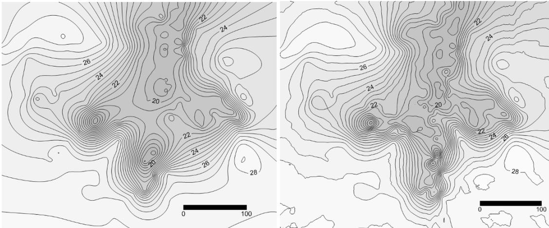
Figure 35: Contour map with the grid generated with 2008 (left) and 2008-9 points (right).
