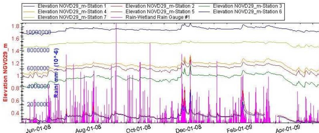
Figure 3: Overview of the water elevation and precipitation at the seven stations in the wetland La Reserva from 5/12/2008 to 5/12/2009.
