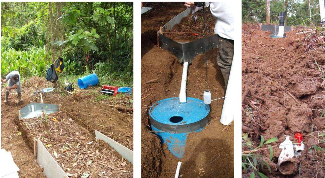
*Runoff plot delineation and isolation from local runoff (left) and system of collecting water (middle) and outlet (right).*
