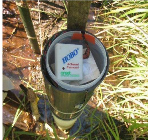
*Hobo data logger in the top's pipe*
