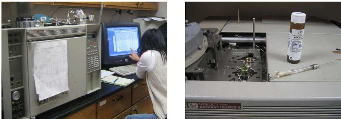
Figure 14: GC/ECD connected to Shimadzu (left) and its injection port (right).
