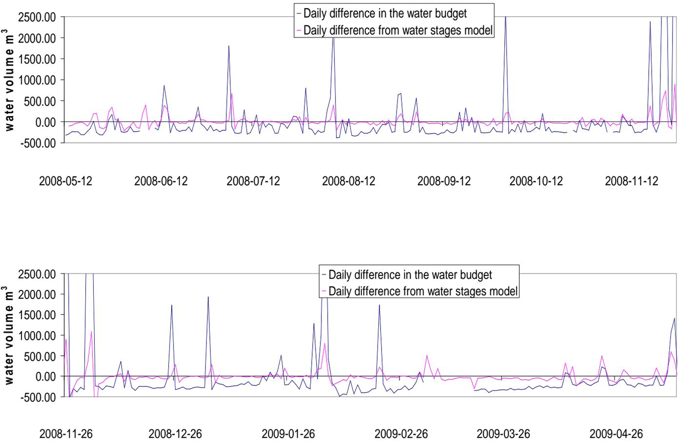
*Figure 41: Comparison between the daily water storage from the water balance and the difference of daily volume from the water stages model.*
