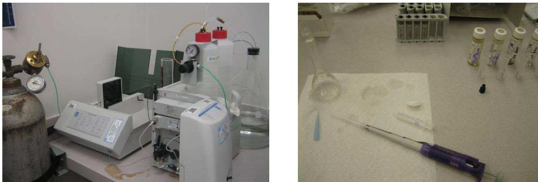
Figure 12: HPLC/EC (left) and preparation of the samples (right).
