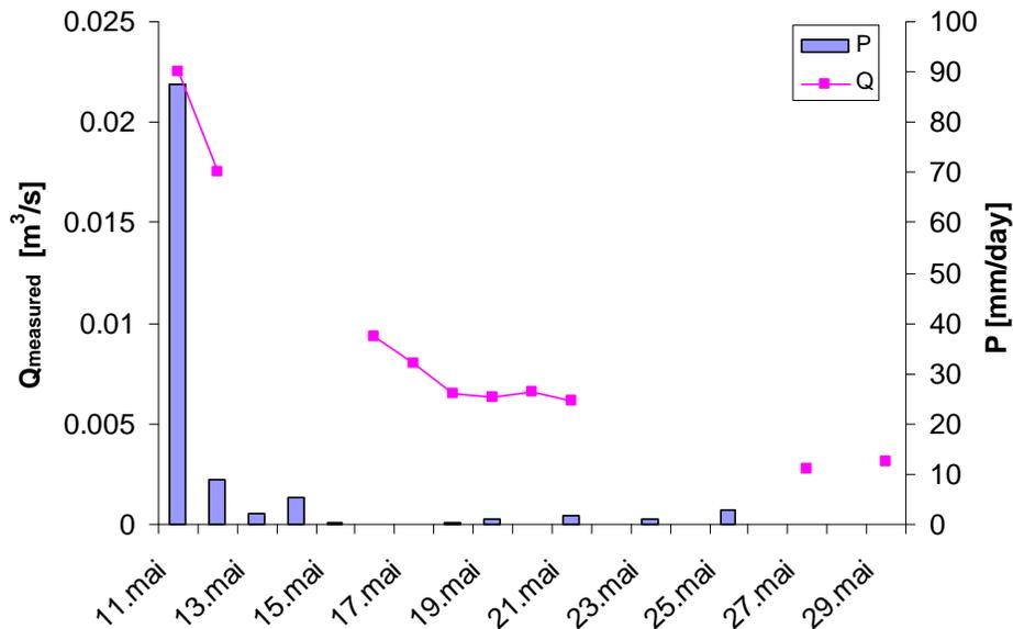
Figure 24: Comparison of the measured flow [m<sup>3</sup>/s] with the daily rainfall [mm].
