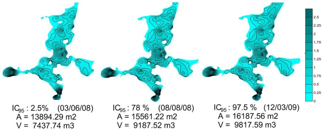
Figure 40: Example of three daily water surface areas and depths representing the most frequent shape (middle) and the lower (left) and upper (right) boundary of the CI<sub>95%</sub>.
