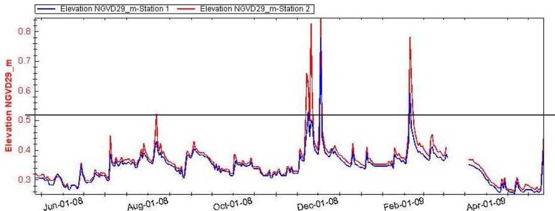
Figure 28: Water elevation upstream (E2) and downstream (E1) of the culvert, May 2008 to May 2009.
