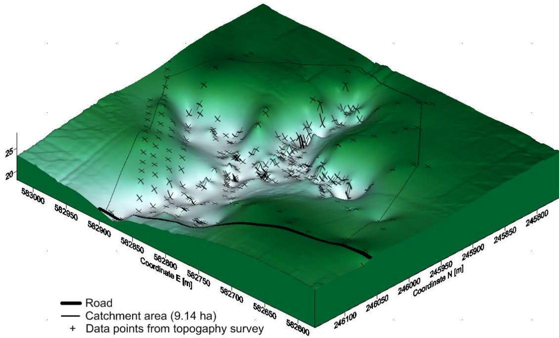
Figure 36: Representation 3D of the topography (grid generated with the kriging method in Surfer) and catchment delineation.
