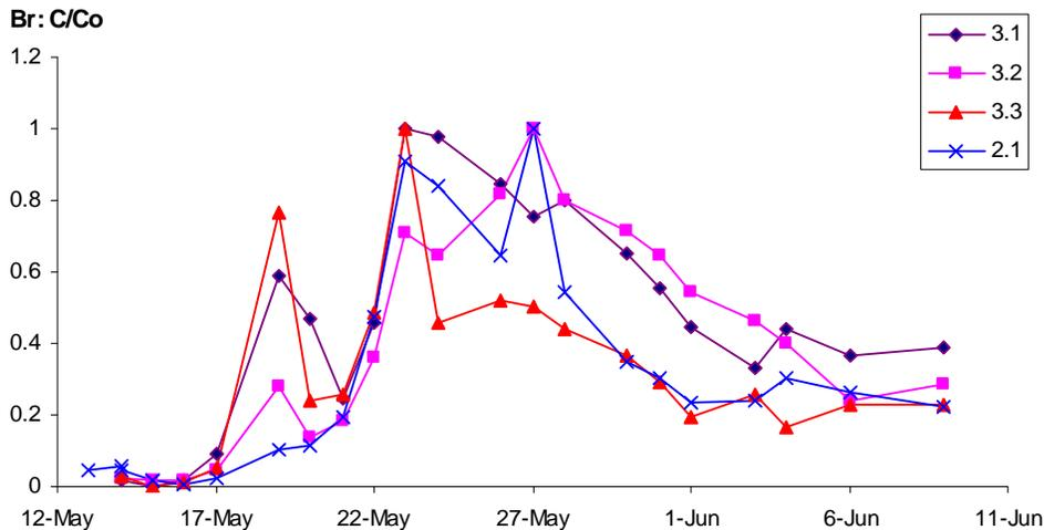
Figure 19: Bromide concentration in the downstream part of the wetland (site 3) and at the outlet (site 2).
