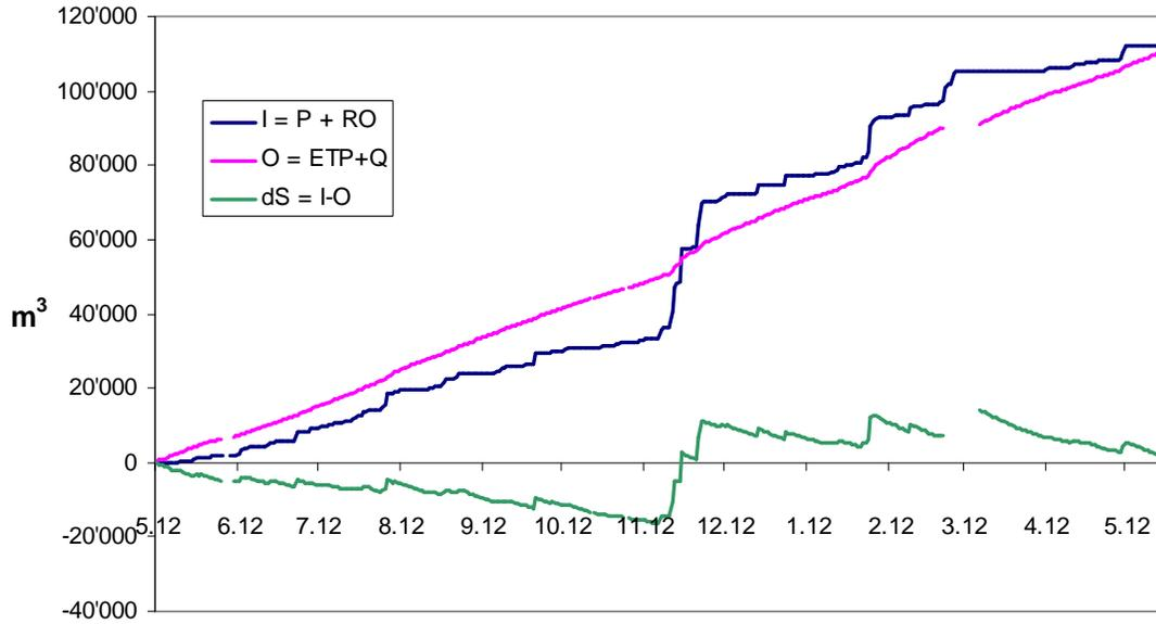
Figure 39: Cumulative water budget [m3] with the evolution of the input (I) and the output (O).
