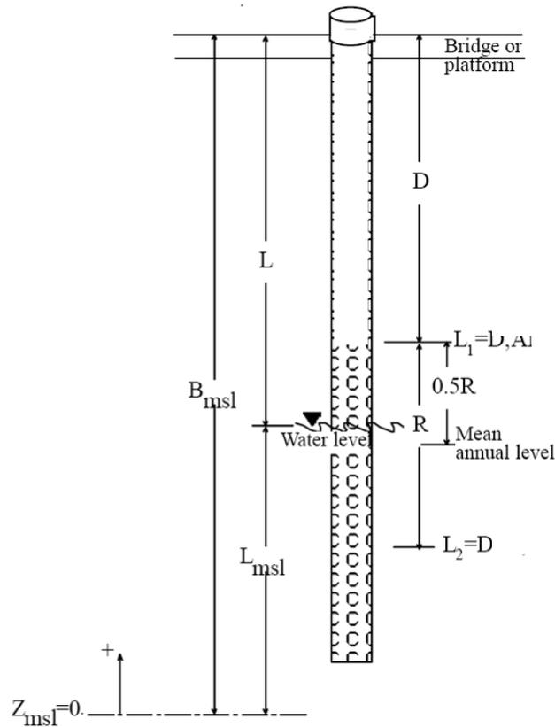
Figure 23: Stage recorder geometry (Source: Schumann and Muñoz–Carpena, 2002).
