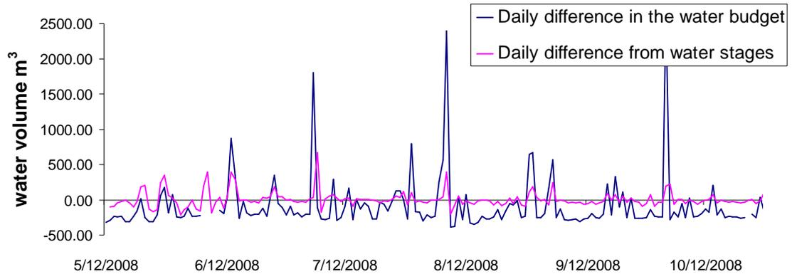
Figure 9: Comparison of the daily difference of volume from the water balance and the water stages model.
