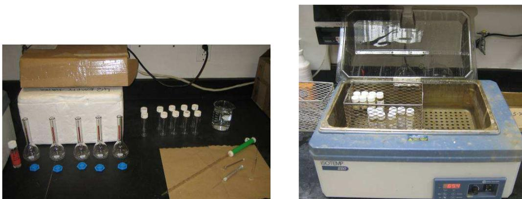
Figure 15: Material to prepare the standard dilution (left) and hot bath (right).
