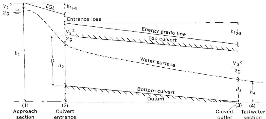
Figure 26: The loss of energy near the entrance is related to the sudden contraction and subsequent expansion of the live stream within the culvert barrel (Bodhaine, 1968).
