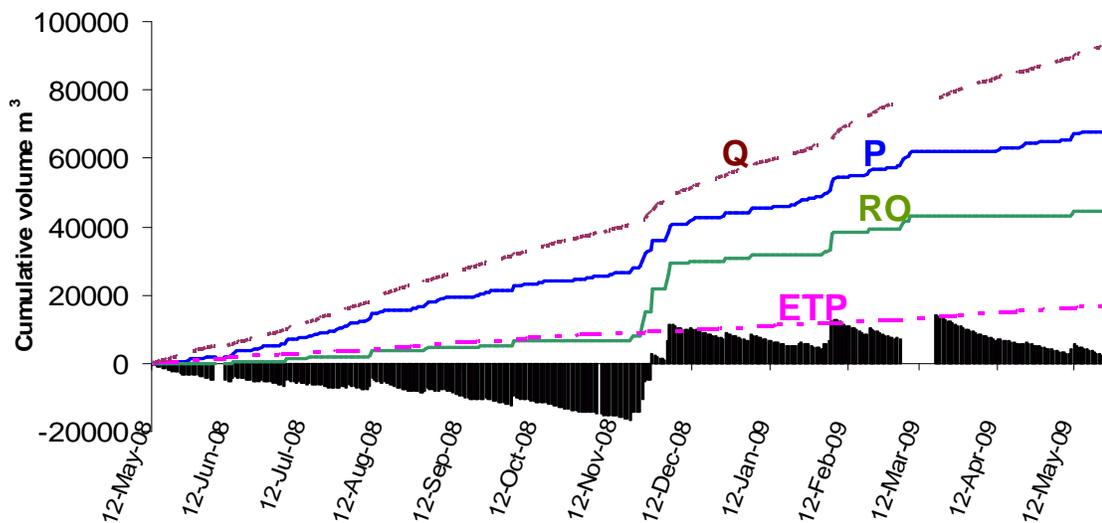
Figure 4: Cumulative water budget [m<sup>3</sup>] over one year with the four key components.
