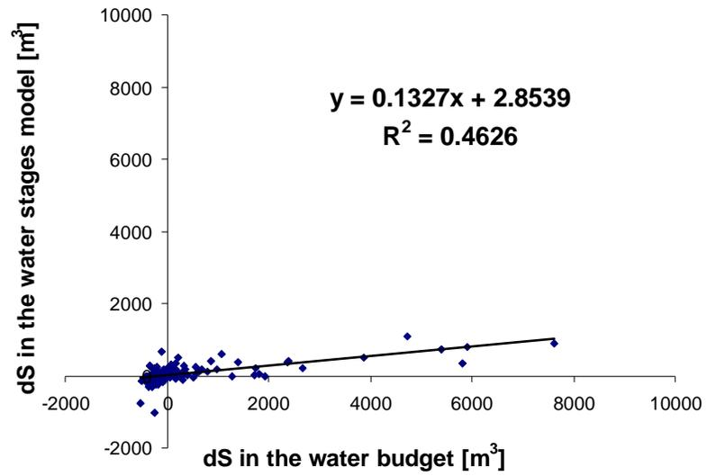
Figure 42: Difference of the daily water storage from the water balance in function of the difference of daily volume from the water stages model.
