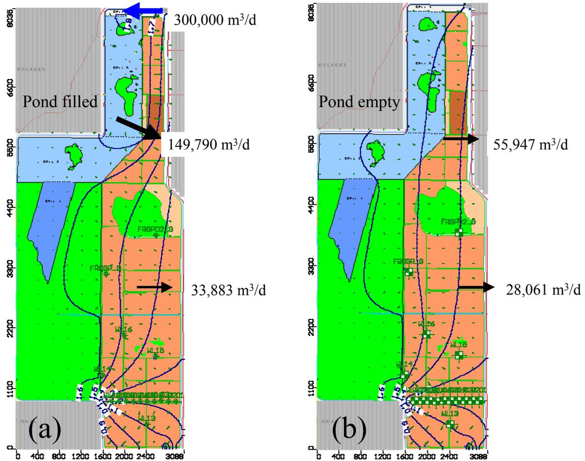
**Figure 11.** Frog Pond Visual MODFLOW simulation results with (left) detention pond filled and (right) detention pond empty (after Morawietz and Muñoz-Carpena, 2003)
