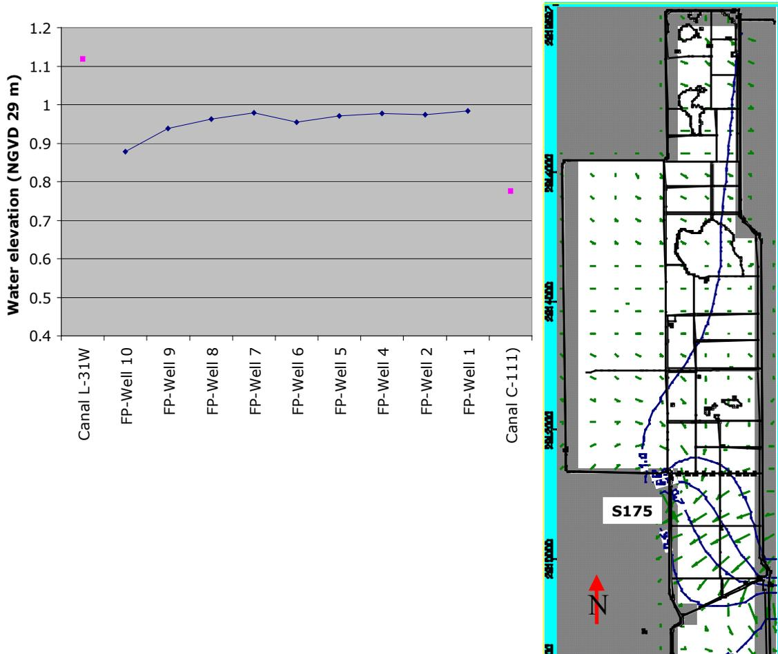
**Figure 10. Steady state groundwater flow modeling to explain anomalous correlation between mean groundwater and canal levels**
