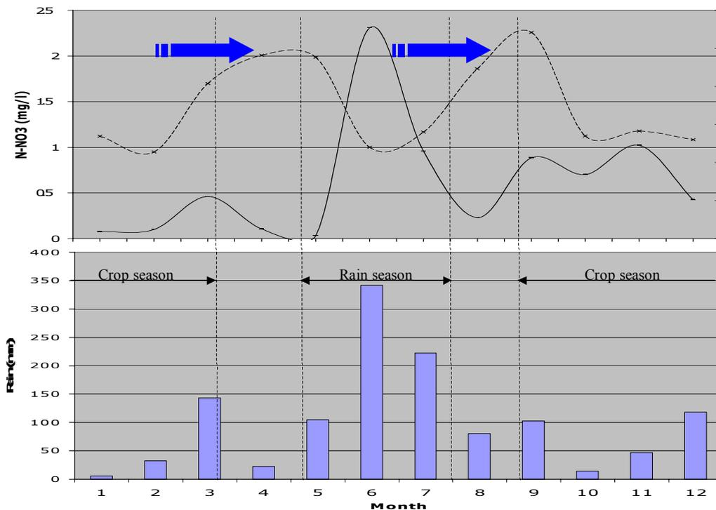
**Figure 15. Annual nitrogen concentrations in ground water samples (the big arrows on top denote chemical reduction of nitrate to ammonia in the groundwater)**
