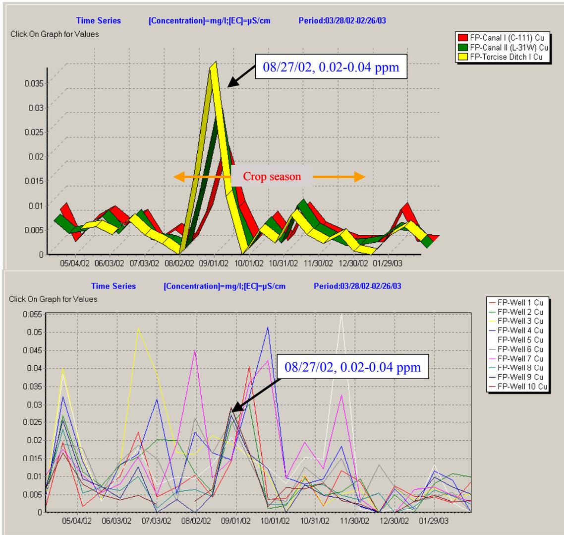
Figure 16. Annual copper concentrations in surface and groundwater samples
