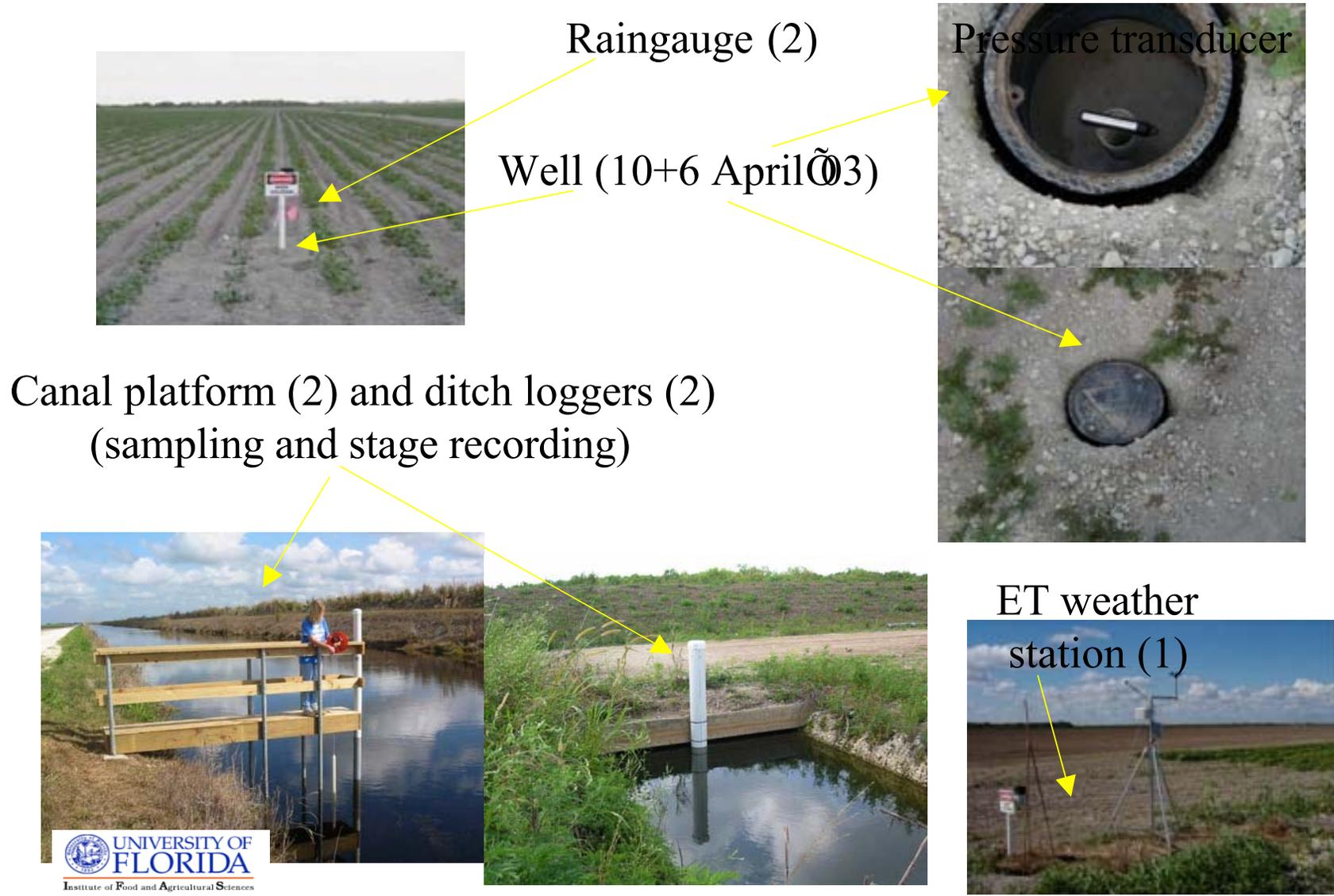
Figure 3. Details of field instrumentation
