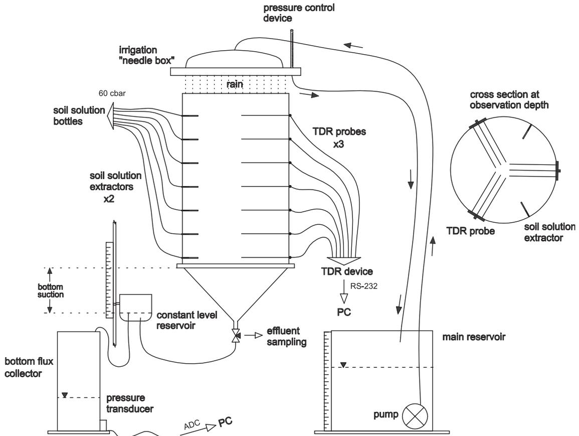
Fig. 3. Transient flow column experiment to test accuracy of the selected  $\sigma_w$ - $\sigma_a$  model.
