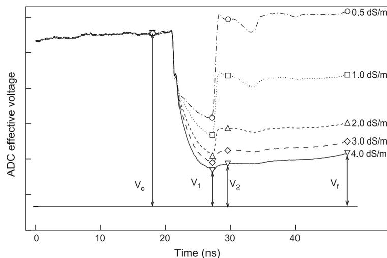
Fig. 1. Experimental results showing the salinity effect on the shape of the TDR curve.  $V_0$  denotes pulse amplitude,  $V_1$ ,  $V_2$  and  $V_f$  are characteristic voltages used to estimate the soil electrical conductivity.
