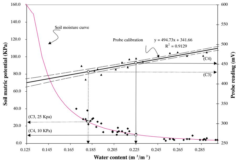
**Figure 4. Soil-water characteristic curve for Krome soil showing irrigation set points for treatments C3 and C4. 95% confidence interval lines for the capacitance probe linear calibration are shown with dashed lines.**
