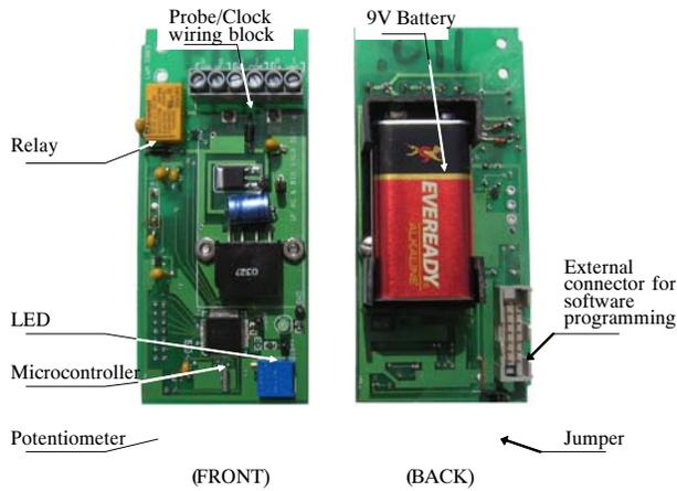
Figure 1. Details of the Quantified Irrigation Controller printed circuit board prototype (front and back).
