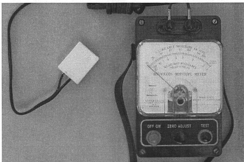
FIGURE 5.10 Gypsum (Bouyoucos) resistance block and reader.
