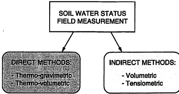
FIGURE 5.1 Methods for measuring soil moisture.
