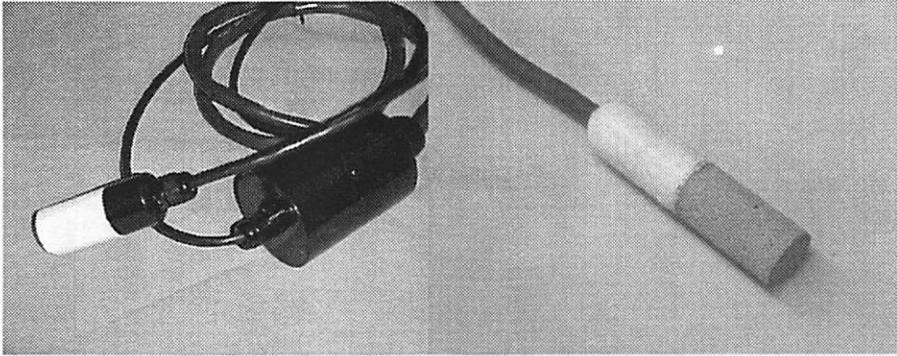
FIGURE 5.12 Heat dissipation sensors.
