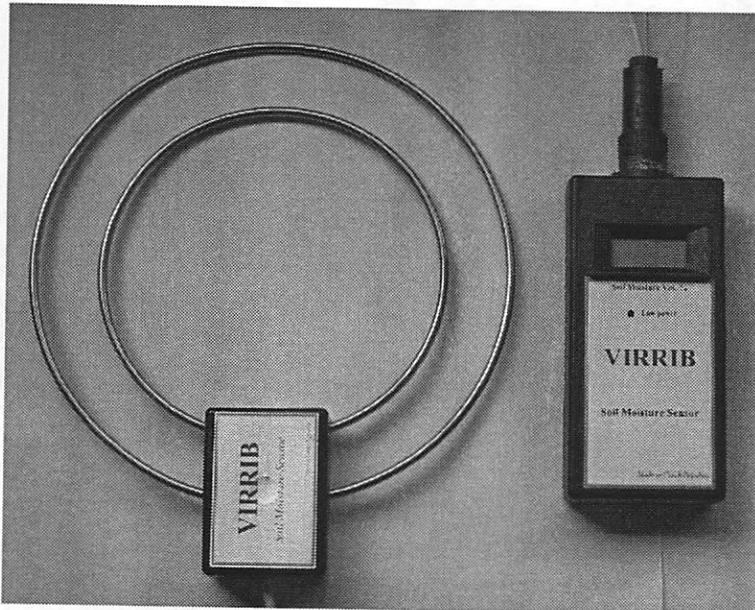
FIGURE 5.7 Phase transmission probe.
