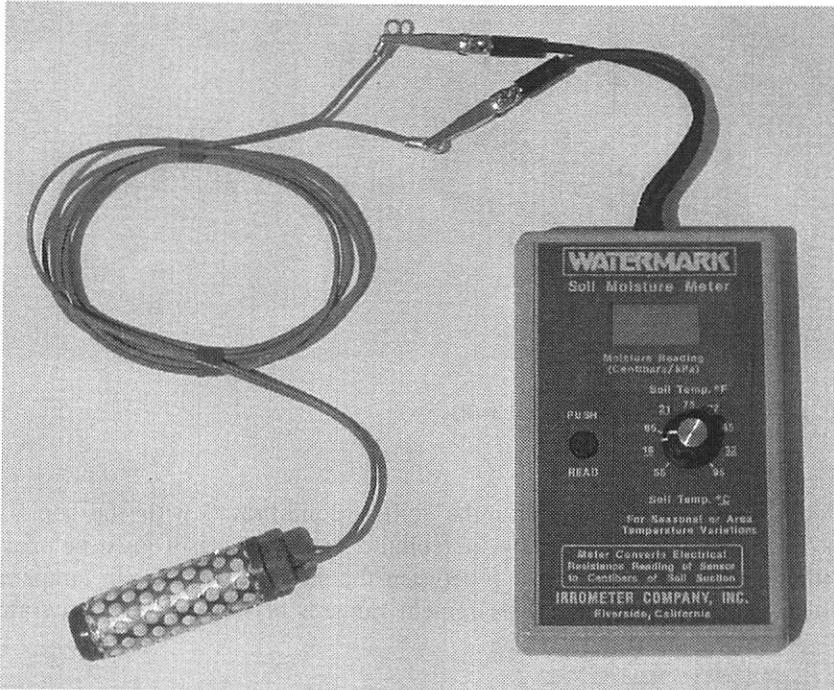
FIGURE 5.11 GMS resistance block and reader.
