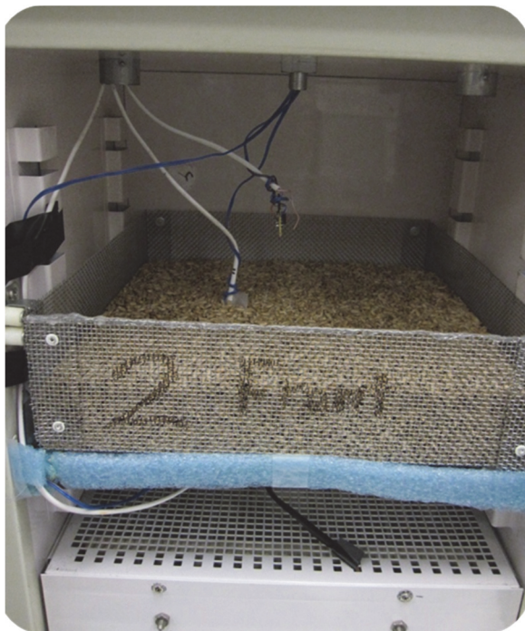
Figure 1. Drying chamber with screen basket.
