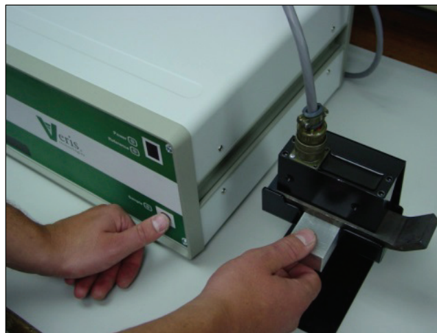
Figure 1. Soil P measurement using a spectrophotometer.
