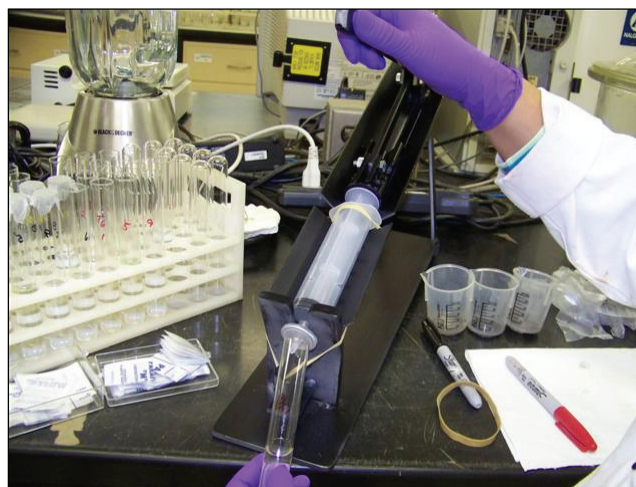
Figure 3. Syringe filter used to test the effects of rapid filtration.
