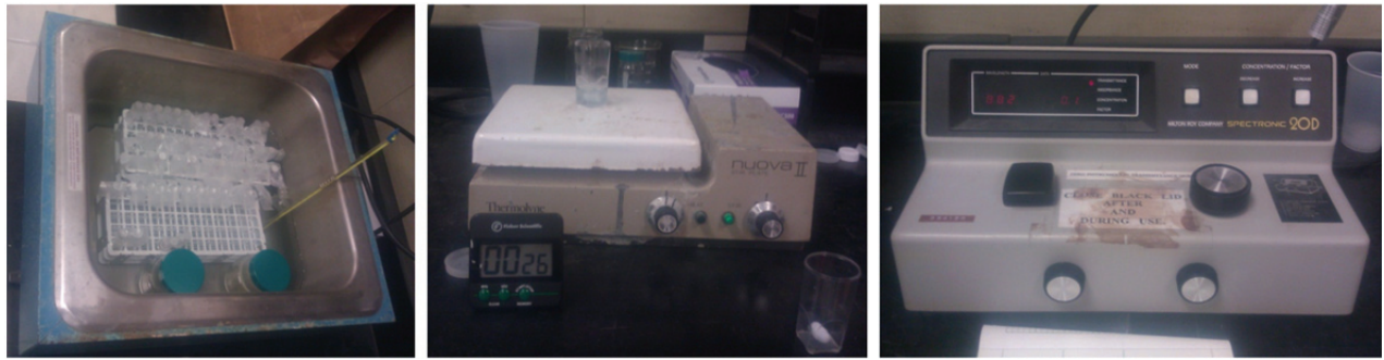
Figure 4. Temperature control bath, stirring plate, and transmittance measurement equipment for the rapid color development method.
