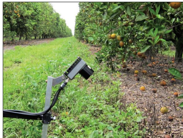
**Figure 2. Downward angle of camera (with metal shield removed).**
