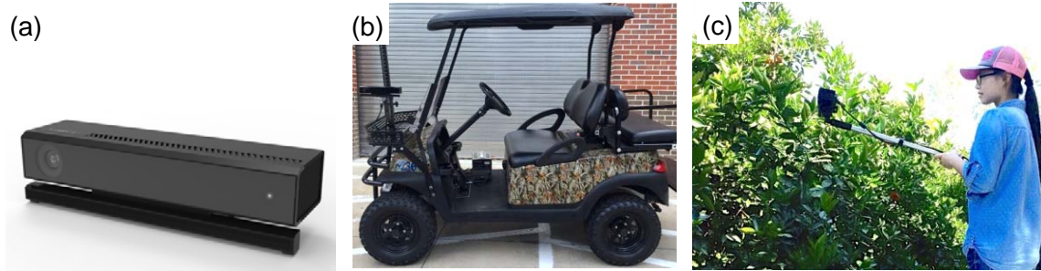
Figure 1. Prototype system for estimating number of small green citrus fruit in the canopy: (a) a camera used to capture images of canopy (Microsoft image) (b) side view of electric cart with a camera and (c) illustration of manual image acquisition.
