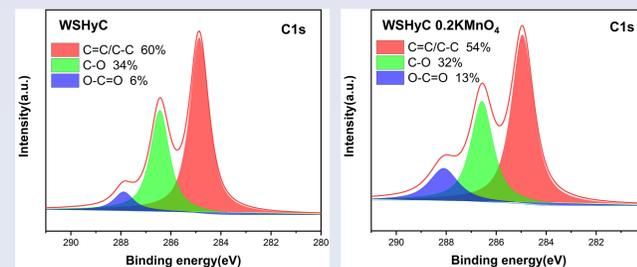
Fig. 5. XPS spectra of C1s of WSHyC and WSHyC-0.2KMnO<sub>4</sub>.
