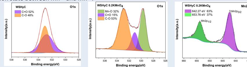
Fig. 6. XPS spectra of O1s and Mn2p of WSHyC and WSHyC-0.2KMnO<sub>4</sub>.
