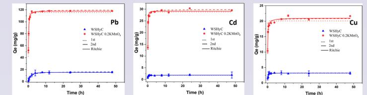
Fig. 7. Sorption kinetics data and fitted models of Pb (II), Cd (II), and Cu(II) onto WSHyC and WSHyC-0.2KMnO<sub>4</sub>.
