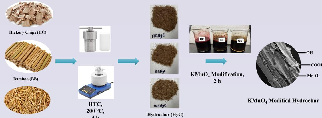
Fig. 2. KMnO<sub>4</sub>-modified hydrochar composite preparation.
