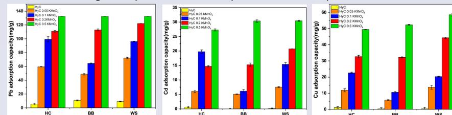
Fig. 3. Effect of feedstock and KMnO<sub>4</sub> modification concentrations on heavy metal adsorption by hydrochar (a) Pb, (b) Cd, and (c) Cu.
