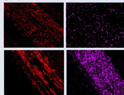
Fig. 4. Elemental mappings of O and Mn of WSHyC (top) and WSHyC-0.2KMnO<sub>4</sub> (bottom), respectively.
