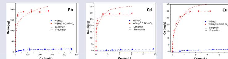
Fig. 8. Sorption isotherm data and fitted models of Pb (II), Cd (II), and Cu(II) onto WSHyC and WSHyC-0.2KMnO<sub>4</sub>.
