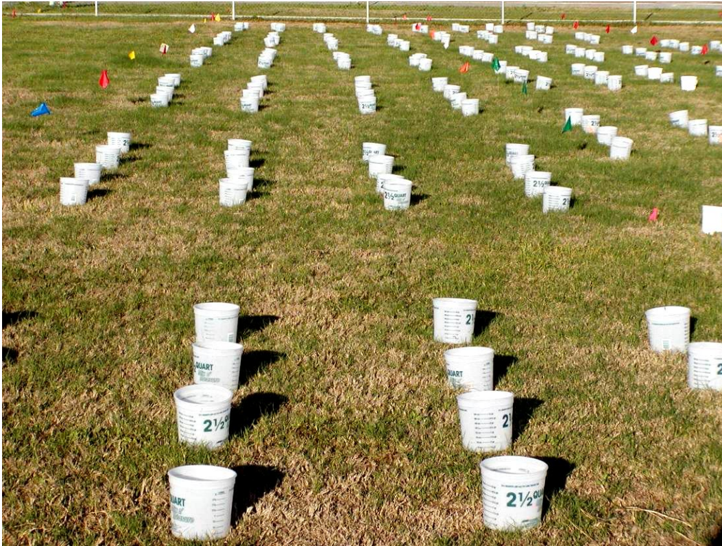
Figure 2-2. Irrigation uniformity distribution test on turfgrass plots.
