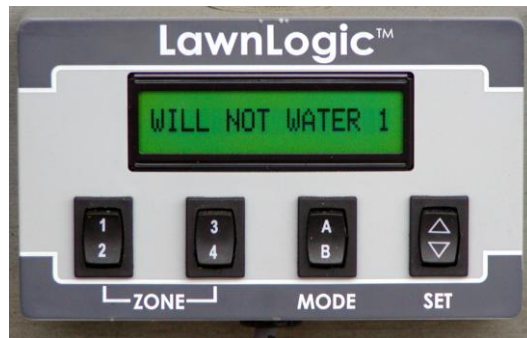
Figure 2-7. Soil moisture sensor-controllers, brands Baseline and Lawn Logic.
