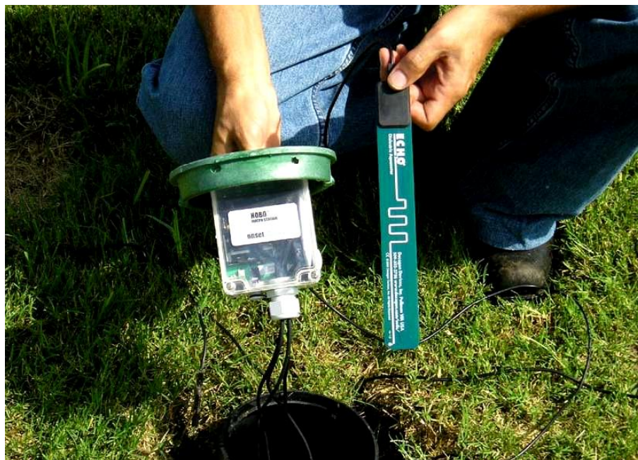
Figure 2-12. ECH 2 O probe, capacitance soil moisture probe shown with a HOBO data logger as installed for this study.
