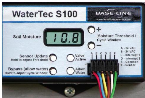
Figure 2-7. Soil moisture sensor-controllers, brands Baseline and Lawn Logic.
