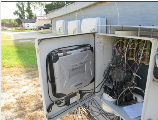
Figure 3. All four ET controllers were wired to circuit boards connected to a laptop running a Visual Basic program that records timestamps of irrigation events. This test was virtual, thus the controllers did not control physical irrigation systems.
