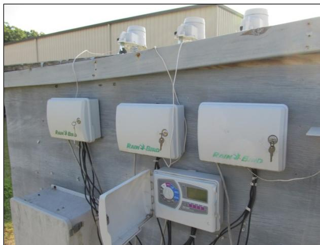
Figure 2. Three ESP-SMT and one ESP-SMTe were programmed to schedule irrigation for multiple configurations of landscape settings possible in central Florida. Each controller had an independent rain gauge (fourth gauge not pictured).
