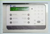
ET Water Smart Controller 100. Signal-based using cellular technology. ASCE method used to calculate ET. Web site used for programming of landscape settings.
