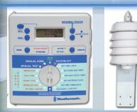
Weathermatic SL1600. Stand-alone design using Hargreaves equation for ET. An on-site weather monitor determines temperature and rainfall. Zip code determines solar radiation.
