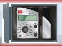
Toro Intelli-Sense. Signal-based using paging technology. ASCE method used to calculate ET. ET is accurate to 1 km<sup>2</sup> of location using MM5 modeling and broadcasted using paging technology.
